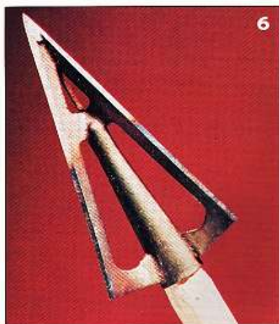
6. Blue edge made by a torch on this Snuffer indicates blade is soft enough to sharpen. 7. Unsharpened Snuffer with rounded edges.
