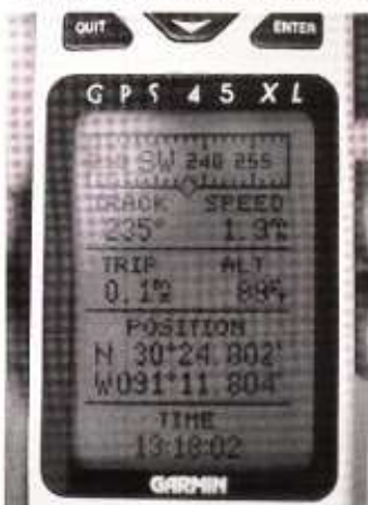
When three satellites have been fixed, a position, altitude and, if moving, direction and speed are calculated.
