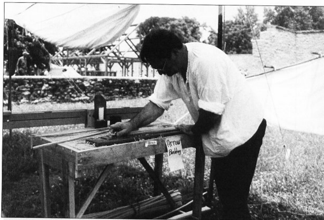
Bob Linksvayer's arrow planing jig consists of two boards cut at 45 degree angles, in which he lays a piece of 1/2 inch square stock and hand planes it to take off the corners. When a shaft is nearly round, he takes it to the die shown at the beginning of this article and pounds it through. He is shown here planing a cottonwood shaft. Cottonwood makes good arrows, but he finds that hickory and ash split easier because they are straighter grained.
