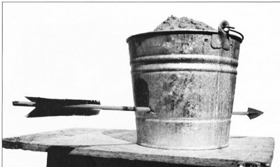
The 200-pound longbow propelled a two-ounce (875 grain) arrow through both sides of a heavy steel bucket filled with sand that had proven capable of stopping all modern, high-powered rifle soft-nosed bullets fired into it.
